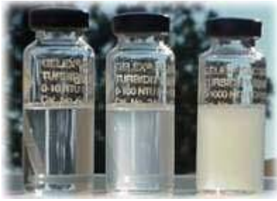
Figure 1.5 Turbidity standards of 5, 50 and 500 NTU (from Wikipedia).
