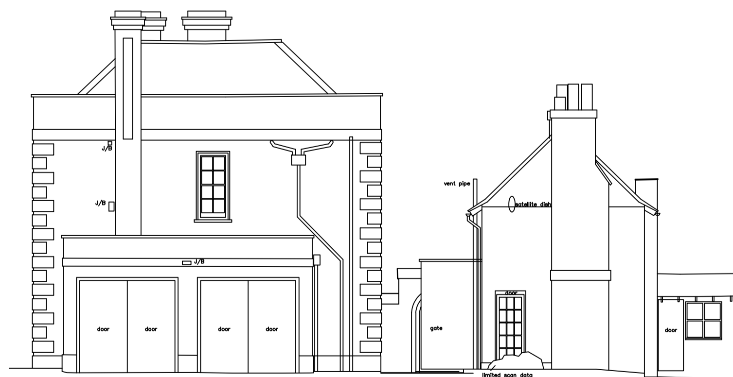
EXISTING EAST ELEVATION (1:100@A1)
